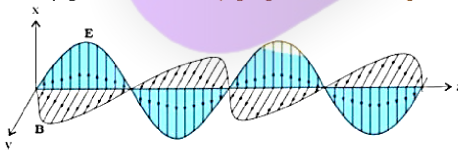
FIGURE 8.4 A linearly polarised electromagnetic wave, propagating in the z direction with the oscillating electric field \mathbf{E} along the x direction and the oscillating magnetic field \mathbf{B} along the y direction.
