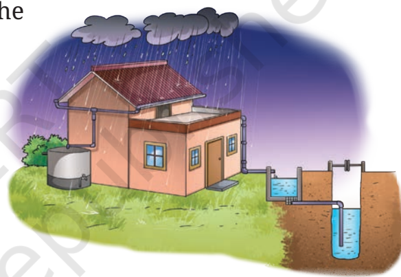
Fig. 11.4 (a): Rainwater harvesting
